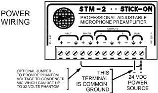
NOTE: THE STM-2 WILL OPERATE (WITH REDUCED HEADROOM) ON SUPPLY VOLTAGES FROM 9 VDC TO 23 VDC.
