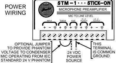
NOTE: THE STM-1 WILL OPERATE (WITH REDUCED HEADROOM) ON SUPPLY VOLTAGES FROM 9 TO 23 VDC.
