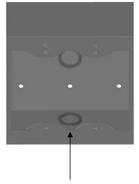
If using conduit, the SMB may be mounted with the knockout facing up or down. The small knockouts fit metric conduits; the larger knockouts fit US conduit.
