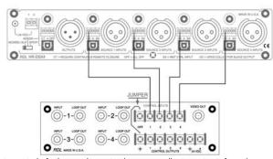
Remote control of other equipment using open-collector outputs from the HR-DSX4; Example shows an HR-DSX4 controlling an RDL RU-VSX4 Video Switcher; A wide variety of OEM equipment can be controlled by an HR-DSX4.
